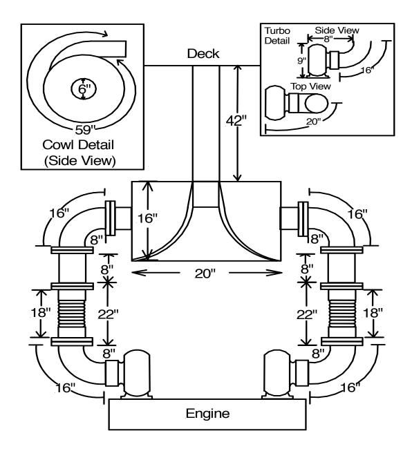
On elbows inside radius and outside radius measurements are best measured from welded seams or flanges.
